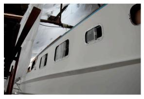
The wheelhouse windows are safety glass, all in good condition and recently re-fitted. There are large 'wind-down' opening windows port and starboard.
