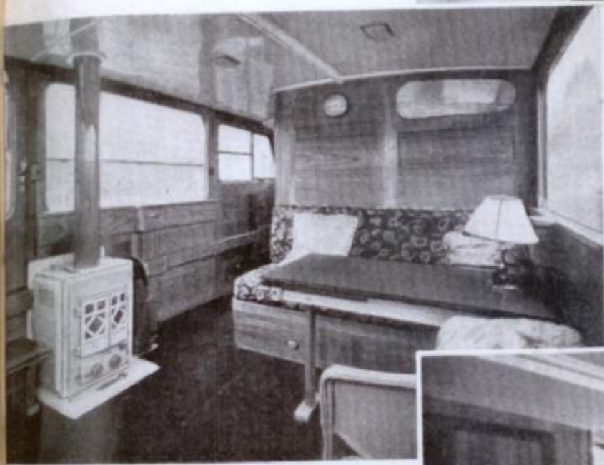
Another view of the saloon. The galley lies beyond the bulkhead. The passageway on the left leads also to the aft stateroom. Note the large drop windows.
